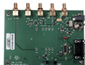
Figure 2. CSAC Developer's Kit includes a powered PCBA with full I/O capability and quick start software. Learn more at http://www.microchip.com/CSAC
